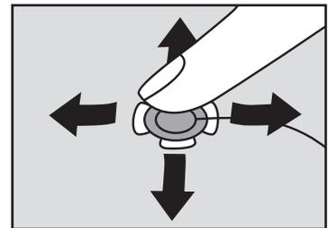
Gently apply pressure with your finger on each of the four leaves around the edges of the electrode.
