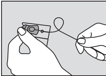
Straighten the lead wire.
